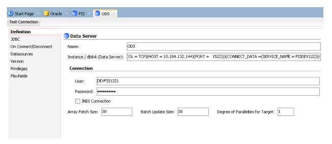
Update the JDBC driver details under Topology→ Physical Architecture→Oracle→ODS and test the connection for the destination schema
