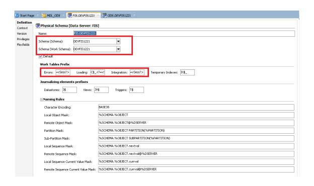
Similarly under Topology→ Physical Architecture→Oracle→ODS→ Definition , update the destination schema details in the Instance/dblink(data server) ,connection User and Password .
